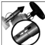
Tighten the shaft screw with an appropriate tool when using the 12" measuring wheel.
