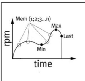
The maximum (highest inflection point), the minimum (lowest inflection point) and the last measured value are saved automatically in the memory. Further values can be captured by pressing the MEM button during the measurement. Certain models can calculate and indicate the average (AV) of these free captured measurement values.
