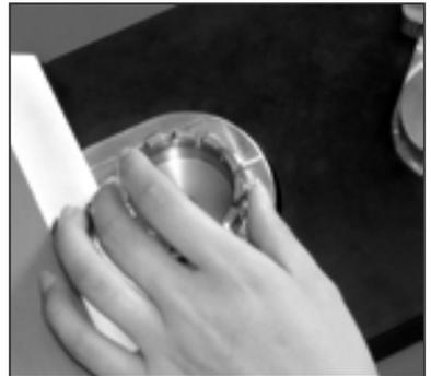
Place the cable connection into the adapter, so that the sleeve of the cable connector stays securely inside the ring and cannot be pulled out through the slot.
