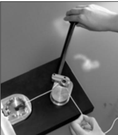
The excentric with the hand lever should be at the home position fully open.
