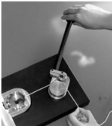
This instrument is designed for measuring tensile strength of soldered or solder-free cable joints with end sleeves, pins, solder pins or similar wire terminal components.
