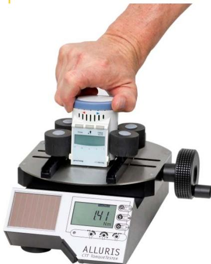
Digital Cap Torque Tester CTT-200 series are particularly suitable as test tools for fast manual torque testing of screw caps, valves, machine components or tools. Objects to be tested (25 - 180 mm diameter) are centrally positioned with retaining bolts and clamped by a contrarotating spindle mounted in the turntable. By manually rotating the test object, the force is transmitted to the torque sensor.
